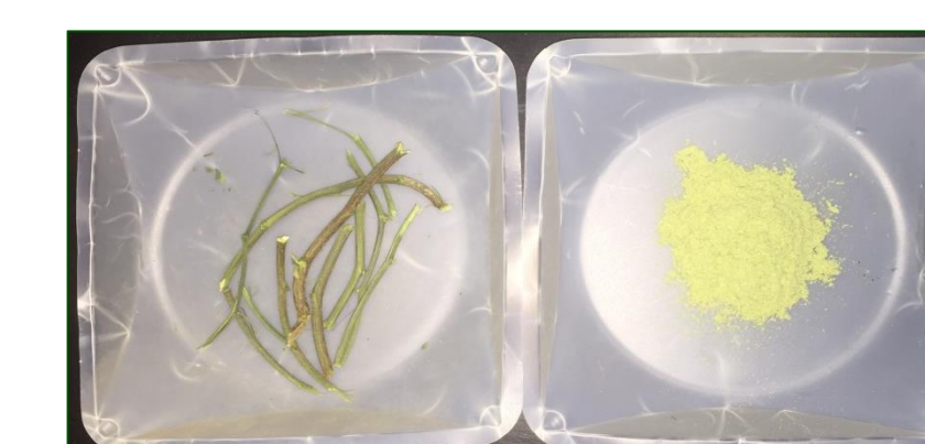
Fig. 4. Ground root and stem samples for iron analysis
